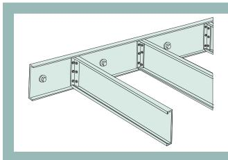
These clips are designed to connect floor joists to the rim joist at the perimeter of the floor, to headers at floor openings, and flush to beams.
