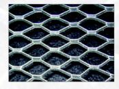
A general all-purpose mesh lath, ideal as a ceramic, concrete base and reinforcement in interior and exterior construction. Easily formed for curved surfaces. The small rigid mesh provides perfect keying of the plaster. The most popular and versatile lath for ceilings, partitions and ceramic tile installation.
