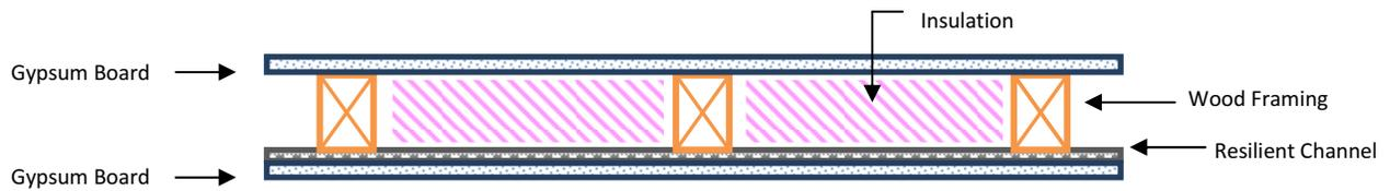
The wall selection chart below illustrates some common types of walls that provide different levels of sound control. This chart demonstrates the effectiveness of the various materials used.
