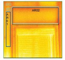
Steel-Framed Home The temperature difference between the insulation (AR01) and the window header (AR02) is  $0.4^{\circ}$ C
