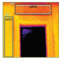
**Wood-Framed Home** The temperature difference between the insulation (AR01) and the window header (AR02) is 1.9°C
