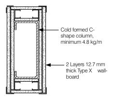
As an alternative to Listed Designs, NBCC Appendix D contains Table D-2.6.1.F. listing the required thickness of Type X gypsum wallboard according to the M/D Ratio of a column. As column fire tests are calculated only on temperature (i.e. failure is determined solely by the temperature of the steel, without any applied load), this Table can be applied to steel columns of any shape or section, including cold formed shapes.
