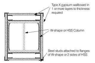
Most Listed Designs for 1h rated W-shape columns utilise no more than two layers of wallboard against the column's flanges (parallel to the web), and one or two layers attached to the steel studs at each end parallel to the flanges. Often, the inner layer is attached directly to the flanges, inside of the studs. Corner beads are required at each corner.
