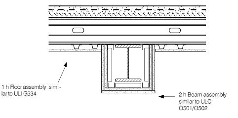
In this example, the construction typified by ULI G534 has been combined with a Beam Design, such as ULC O501 or O502. Alternatively, the same result can be achieved by using ULI L524. In each of these cases, the actual construction details vary between the Designs, and the designer must select the most appropriate.
