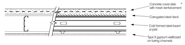
\* Slab to be mininum thickness as specified in selected Listed Design, or else 50 mm (NBCC Table D-2.3.5.).
