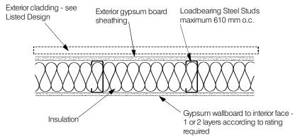
If the wall falls under the NBCC Limiting Distance requirements (Subsection 3.2.3.), then both the insulation and the exterior cladding must satisfy Article 3.2.3.7., Sentences (1) to (9) as appropriate. Many Designs also require some form of lateral support or bridging, by such means as horizontal steel straps or channels.
